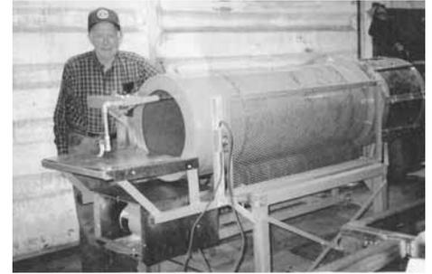
**Belt-driven rollers turn the cleaner, with power supplied by a 3/4 hp electric motor.**
