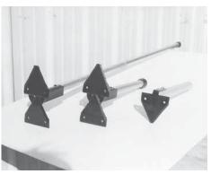
Terry Morgel makes garden hoes from used sickle sections. Two hoes have double sickle sections welded to a large flat washer.
