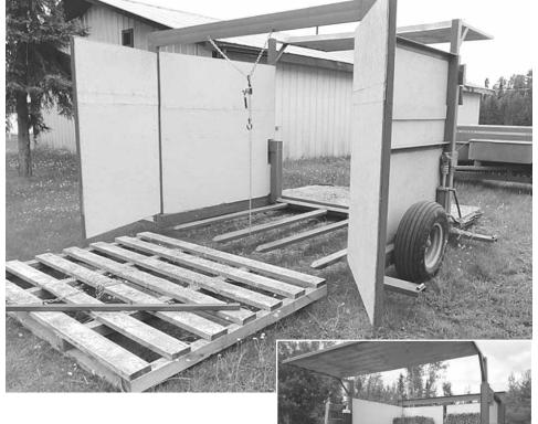
Pallet slips over 4 long forks to form cart's floor. After bales are loaded, Keddie lowers forks to ground, then drives forward to leave pallet in the field.
