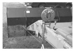
Attached to loader arm, homemade tilt gauge lets Clifford Tonsfeldt see the bucket angle at a glance when digging or picking up material.
