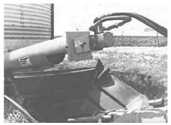
Hydraulic drive easily installs on most any existing unloading auger without removing the bearing.
