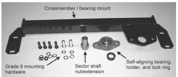
Installation of stabilizer requires no drilling. It provides support to steering sector shaft and eliminates sector shaft play in steering box.
