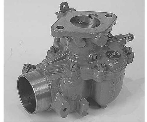
**Gary Hoefling says his modified Zenith carburetor cleans up the black smoke and fouled spark plugs common to Deere 3010/3020 and 4010/4020 tractors.**
