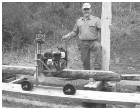
Cal Reed stands beside a board he cut with the Lumber Smith Sawmill. At 105 lbs., the Lumber Smith is the lightest weight band sawmill in its class.
