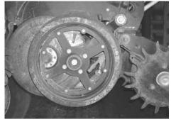
Open spoke design of new replacement gauge wheels keeps them free of mud.
