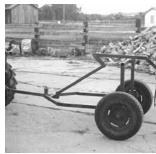
Innovative log arch pins to tractor drawbar and uses its own tongue to lift front end of log off the ground.
