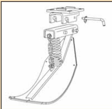
The Quick Disconnect makes efficient work of installing/removal of the STALK STOMPER devices for storage and transport of your combine head. May Wes's STALK STOMPER has a non-stick UHMW poly surface that reduces mud and debris build up and provides for virtually a maintenance-free operation. Its rugged heavy-metal construction withstands extended wear. The May Wes STALK STOMPER'S springs maintain down pressure on the stalks whenever your combine head is in the operating position.
