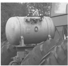
Propane Enhancer injects a little propane into diesel engines for faster speeds, more power, and a cleaner burn in tractors and trucks.
