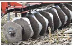
The flat sides on Falk's 5-sided disk blades push crop residue down into the soil surface. Only the points penetrate the soil.
