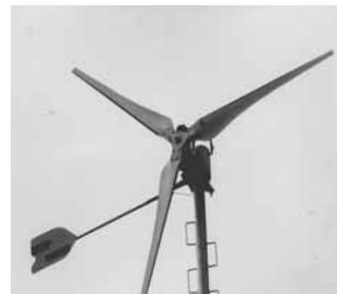
**Win-Pressor turbines are designed to produce compressed air instead of electricity. Photo upper left shows unit in gear. Photo lower left shows unit furling and out of gear.**
