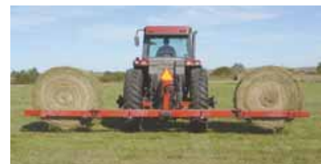
Two Banger bale accumulator picks up 2 bales, one on either side of tractor.
