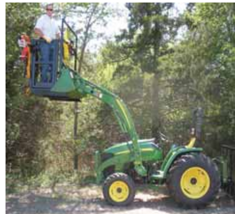
“Bucket Basket” provides a safe work platform with work space for 2 people.
