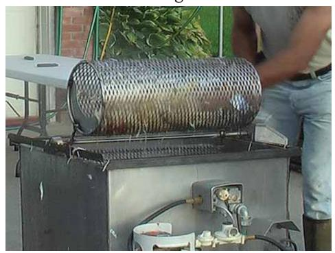
Two stainless steel baskets hold 20 to 30 lbs. each. They're turned by a light-duty motor, providing a more consistent scald since only half the birds are in the scalder at any one time.
