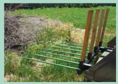
"Ultra fork" clamps onto loader bucket and comes with 7 replaceable, 32-in. long spears. Top part of frame has 4 stake pockets to hold 2 by 4's that form a "backstop" when hauling brush.
