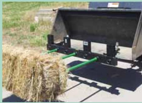
"Ultra fork" clamps onto loader bucket and comes with 7 replaceable, 32-in. long spears. Top part of frame has 4 stake pockets to hold 2 by 4's that form a "backstop" when hauling brush.
