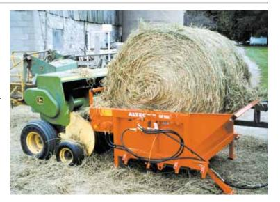
doesn't break up the hay but instead gently unwinds it. The legs are needed only if the baler's pickup reel is more than 2 ft. off the ground. And when you're done using the unwinder to make small square bales, you can remove the legs and use it as a normal bale unwinder to deliver feed into bunks or onto pasture ground."
