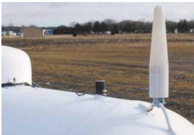
**Alarm attaches to lifting lug on tank. It lights up when tank gets down to 25 percent full.**
