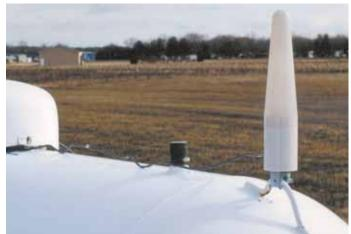
Alarm attaches to lifting lug on tank. It lights up when tank gets down to 25 percent full.
