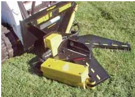
**Model HTC-14 can cut a 14-in. tree at ground level in 5.5 seconds. All major pivot points are machined and greaseable for long life.**
