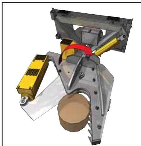
With the push of a button, Timberline™ Tree Shears rotate up to 110 degrees from horizontal.
