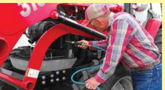
Wand tubing on the Radiator Genie is small enough so you can get into confined areas, yet big enough to create a lot of force with air or water.
