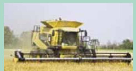
**AWS air reels are available to fit all makes of combine headers. The curtain of air created by the manifold system across the front of the header provides an even flow of crop material into the combine with less damage.**
