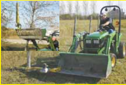
Hydraulic-powered cutter attaches to loader bucket.
