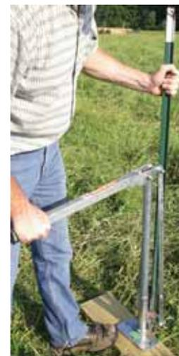
JackJaw grabs the post using a pair of cam-shaped, case-hardened steel jaws.
