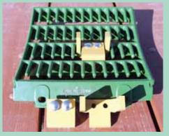
"The problem with the standard round bar concave in the Deere STS rotor is that there isn't enough space between the round bars to let grain out," says Estes. "We have designed a new grate that has 1/2-in. square keys installed instead of the round bars, with a 1 1/2-in. space between them for 68 percent greater openings."
