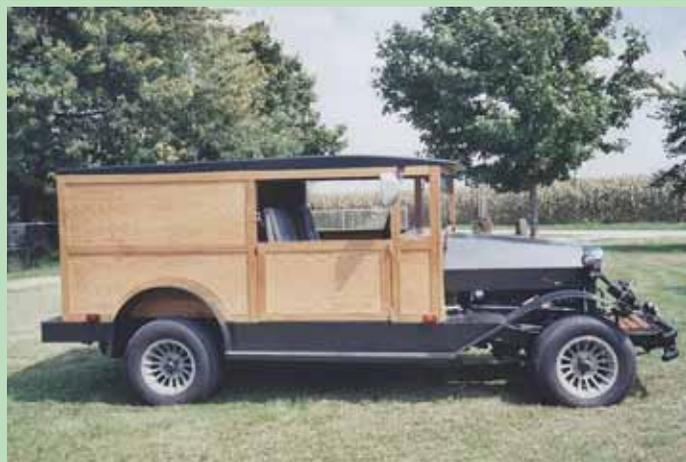
Van's unibody construction made it easy to strip down and then rebuild with a rollbar framework and real wood exterior.
