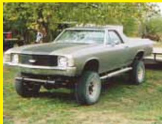
When the body rusted off my 1975 Chevy 4-WD shortbed pickup, I replaced it with the body from a 1971 Chevy El Camino car. I had to build 8 new body mounts. It works perfect and turns a lot of heads. **(Shane Myrick, 17758 Vail Rd., Pleasanton, Kan. 66075, ph 913 757-3309; cell 913 671-9812)**
