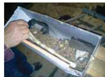
Seed tube "stoppers" consist of three 1/2-in. dia. pvc pipes with fittings on them. To plant, Stutzman moves handle up and down to force stoppers in and out of pipes.
