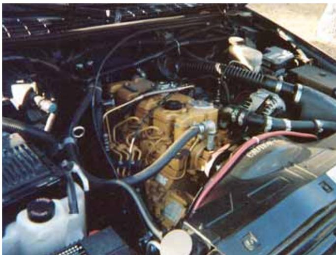
To convert his Chevy S-10 pickup to diesel power, Jeff Flicek matched up a new 2.2L 3024T Caterpillar diesel engine to a Chevrolet 700R4 automatic transmission.
