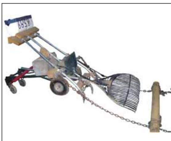
Planter has three 1-in. dia. metal pipes attached to 4-wheeled truck dolly at an angle. Upper end of pipes extends a short distance into mailbox.
