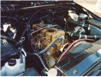
To convert his Chevy S-10 pickup to diesel power, Jeff Flicek matched up a new 2.2L 3024T Caterpillar diesel engine to a Chevrolet 700R4 automatic transmission.
