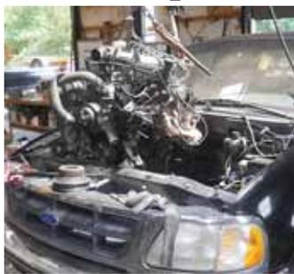
Truman Miller repowered a 1997 Ford F-150 with a 5-cyl. Deutz diesel engine that he bought on Craigslist for \$1,500.
