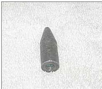
Tapered tip fits onto end of Jim Rankin's grease gun so he doesn't have to take the dust cap off the wheel hub to lubricate it.
