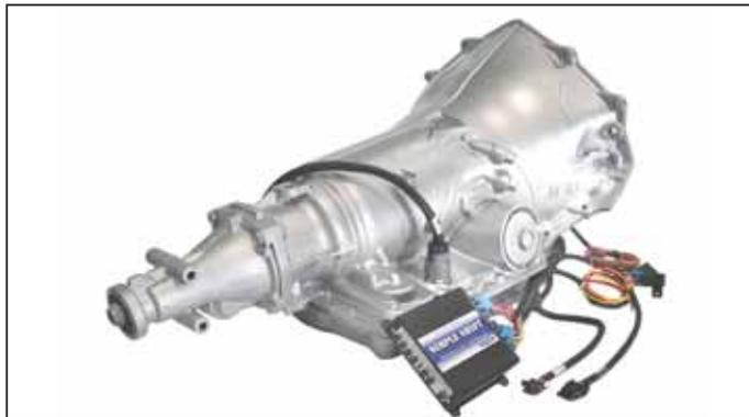
Simple Shift Transmission Controller lets an electronic overdrive shift smoothly whether it's under load or not, at lower rpm's and with better fuel efficiency.
