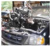
Truman Miller repowered a 1997 Ford F-150 with a 5-cyl. Deutz diesel engine that he bought on Craigslist for \$1,500.
