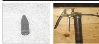
Tapered tip fits onto end of Jim Rankin's grease gun so he doesn't have to take the dust cap off the wheel hub to lubricate it.
