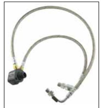
Simple bolt-on kit eliminates “deadhead” problems in 1999 through 2003 Ford Powerstroke engines.
