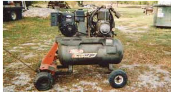
Gas-powered air compressor is mounted on the front axle and frame of an old riding mower.
