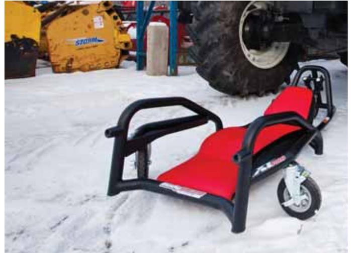
The frame on this heavy duty floor creeper is built strong enough to withstand the weight and impact of a falling vehicle.
