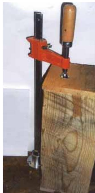
Kit holds clamp on work bench so it can be used to secure tall objects in place.
