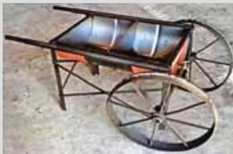
**Tim Renger, Bancroft, Iowa:** "Changing oil on my 4-WD tractor was always one of the messiest and most back-wrenching jobs on the farm until my friend Mark Bauer came up with this two-wheeled oil caddy. Now I can wheel the cart under the tractor, reach under to remove the plug and drain the oil without spilling a drop."
