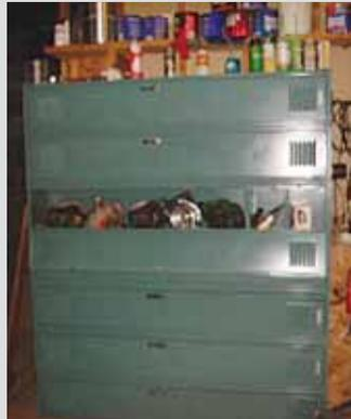
**Bud Roenigk, Cabot, Penn.:** "I needed an inexpensive storage unit for my shop tools, such as saws and drills. I found a set of metal lockers that had been removed from a school during renovation. I stacked the lockers on their sides so the doors open down. My tools fit neatly into the lockers, and my cost was minimal."
