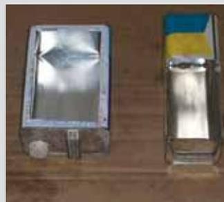
**Bill and Karen Hinckley:** "Empty 1-gal. metal cans can be used to make convenient bolt or parts bins. I use a knife to cut an opening in one side of the can and then bend the edges over to eliminate the sharp edge. Sometimes I cut the opening into one of the narrow sides of the can so it won't take up as much room on a shelf. I use this idea to store parts when restoring a tractor, labeling each can with a piece of tape."
