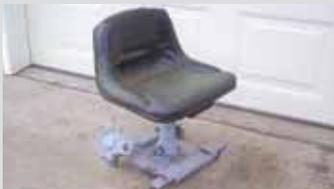
"The stool rides on four small caster wheels. I used the seat and mounting frame from an old Sears riding mower, welding it on top of a screw jack off a Toyota car. The bottom of the jack is welded to a steel plate. The seat adjustment mechanism consists of a sprocket with an eyebolt welded onto one of the cogs."
