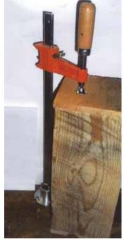
Kit holds clamp on work bench so it can be used to secure tall objects in place.
