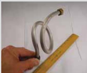
**Ken Brading, Atascadero, Calif.:** "In your last issue, a reader told how he bends thin wall tubing by filling it with sand and plugging both ends to keep it from collapsing."
