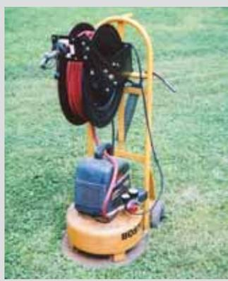
**Edward Miller, Batavia, N.Y.:** "This is the handiest tool I've ever built for around the farm. I mounted a new compact air compressor on a 2-wheel hand truck and bought a new hose reel to mount above it. I can take it anywhere and run the hose out as needed. I've also got a hook on back to hold a grease gun."
