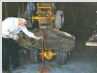
chain hoist from the trusses in my pole barn. It's really handy for sharpening the mower's blades. I place a safety stand under the deck and then let the tractor down until it rests on the stand. Then I can sit in a chair and sharpen the blades without having to remove the deck or bend over."
