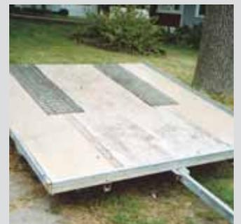
**Rex Gogerty, Hubbard, Iowa:** "Discarded tracks from an old crawler tractor, screwed to the floor of a flatbed trailer, can provide extra traction for loading 4-wheelers, garden tractors and skid loaders. My son found the tracks in a junk yard."
