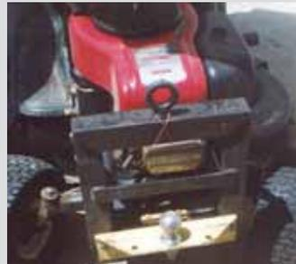
**Bill Reeks, Cromwell, Ky.:** "I used 2-in. angle iron to build a 'push frame' on front of my Sears Craftsman garden tractor. Metal braces extend from the top of the frame down at a 45 degree angle to the tractor frame. I attached a 1 7/8-in. ball hitch to it that lets me push small trailers around without having to look backward, which helps a lot because I have arthritis in my shoulders and neck. In fact, I've mounted push frame-mounted ball hitches on several garden tractors."
