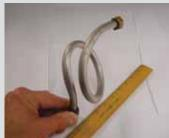
Ken Brading, Atascadero, Calif.: "In your last issue, a reader told how he bends thin wall tubing by filling it with sand and plugging both ends to keep it from collapsing.
