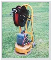
Edward Miller, Batavia, N.Y.: "This is the handiest tool I've ever built for around the farm. I mounted a new compact air compressor on a 2-wheel hand truck and bought a new hose reel to mount above it. I can take it anywhere and run the hose out as needed. I've also got a hook on back to hold a grease gun."
