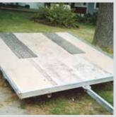
**Rex Gogerty, Hubbard, Iowa:** "Discarded tracks from an old crawler tractor, screwed to the floor of a flatbed trailer, can provide extra traction for loading 4-wheelers, garden tractors and skid loaders. My son found the tracks in a junk yard."
