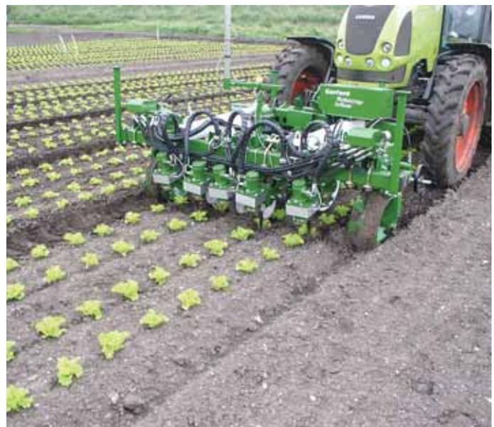
Robocrop cultivator uses GPS guidance to chew through weedy fields at 12 mph, working to within half an inch of the row and weeding between plants in the row.
