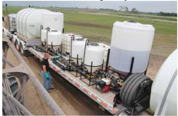
Mike Elsen built this "supersized" liquid spray tender on a 50-ft. spread axle drop deck trailer. He tows it with a 475 hp semi tractor equipped with a tag axle.
