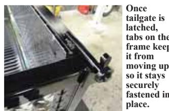
Once tailgate is latched, tabs on the frame keep it from moving up so it stays securely fastened in place.
