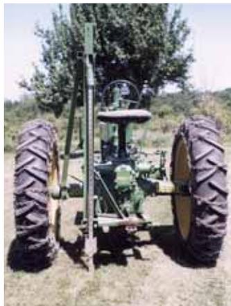
Glen Hall used scrap metal to build this steel post driver that mounts on back of his 1939 Deere B tractor.
