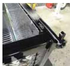
Once tailgate is latched, tabs on the frame keep it from moving up so it stays securely fastened in place.
