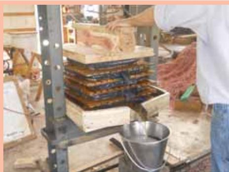
The shredded apple pulp is put into Miller's 24-in. square press made from oak and lined with stainless steel.
