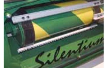
Feederhouse slats attach to reinforced rubber belts instead of metal roller chain.
