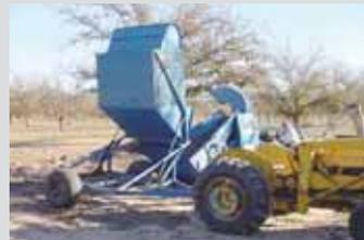
Pecan dump trailer was built using the wheels, axle and dump basket from a peanut harvester.
