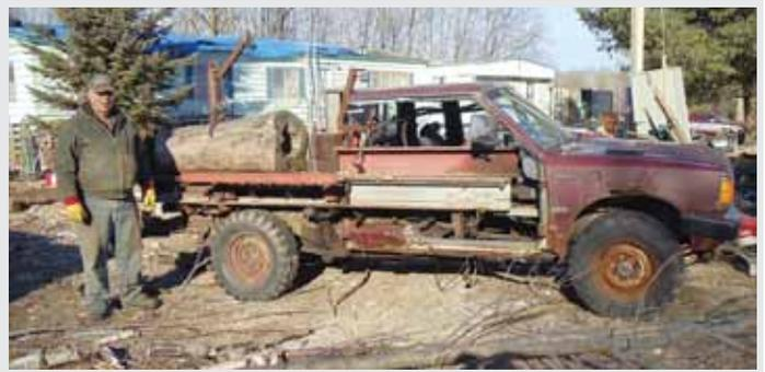
Richard Thompson converted an old Datsun pickup into this self-propelled splitter. He uses it to make 4-ft. log sections for his outside furnace.
