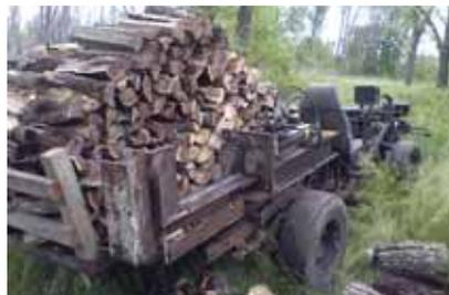
Rear view of Clayton Otwell's self-propelled log splitter shows firewood stacking bed that makes it easy to haul wood back home.
