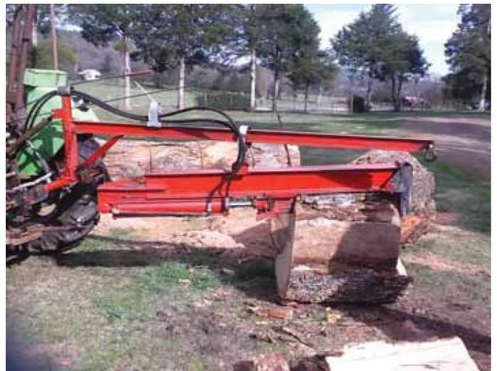
Larry Zenz's 3-pt. mounted splitter is free to swivel 360 degrees under a 7-ft. long, 3-in. I-beam arm. It allows him to split logs no matter what direction they're laying.
