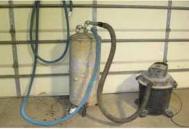
Shop vac sucks water into 20gal. pressure tank. When tank gets full operator shuts off shop vac, then opens shut-off valve on tank to drain water onto ground.
