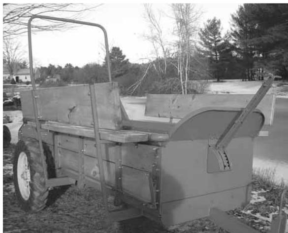
Ed Lavigne converted this old Deere L51 manure spreader into a wagon to carry people on hay rides. A set of stairs can be raised or lowered from the tractor seat.
