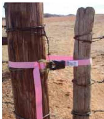
Ratchet strap helps open and close gates secured by tight wire loops. You place strap under wire, then tighten ratchet until wire is loose enough to remove.
