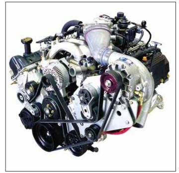
Vortech Engineering, known for its horsepower-boosting superchargers for high performance race cars, has started adapting products to fit stationary engines used by farmers. Photo shows a Ford V-8 engine equipped with a Vortech Supercharger.
