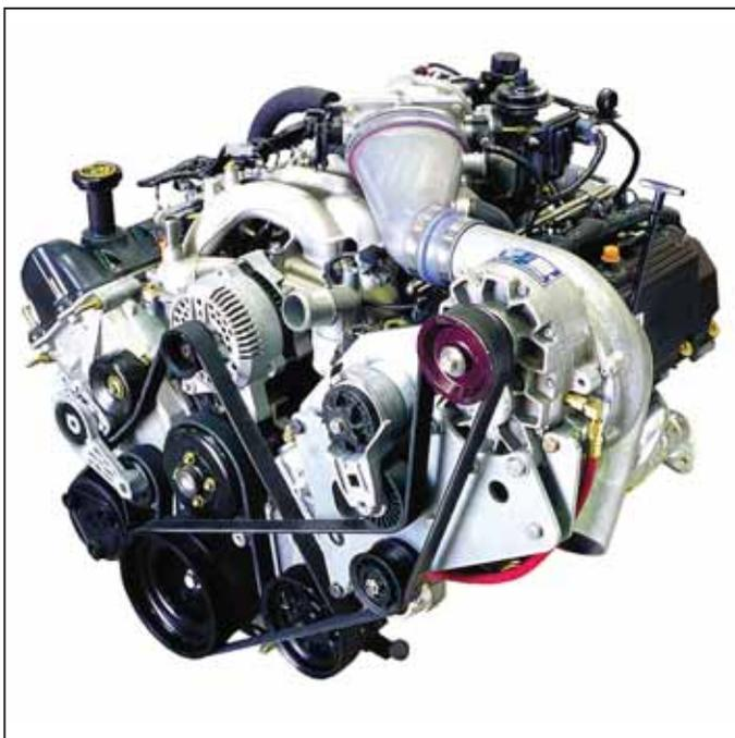
Vortech Engineering, known for its horsepower-boosting superchargers for high performance race cars, has started adapting products to fit stationary engines used by farmers. Photo shows a Ford V-8 engine equipped with a Vortech Supercharger.
