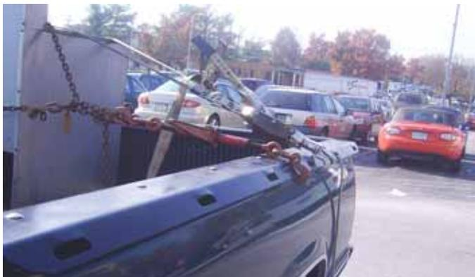
New tie-down rail bolts onto the side rails of any shortbed or longbed pickup, except ones equipped with dually wheels. Inventor Dennis Baker says the system can be used with everything from tractor-trailer tie-downs to nylon straps and come-alongs.
