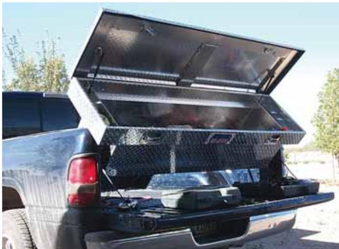
A handheld remote is used to bring toolbox to back of pickup where it tilts for easy access.
