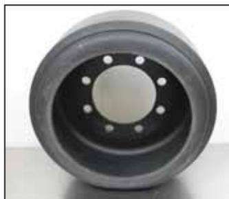
Polyurethane bogie wheels are said to work better than steel or rubber, both on the road and in the field.
