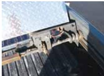
Bicycle sprockets mount on a shaft that's driven by an electric winch. Sprockets "walk" along lengths of chain mounted on rails.
